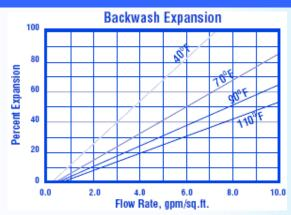
**Backwash:** After each cycle the resin bed should be backwashed at a rate that expands the bed 25 to 50 percent. This will remove any foreign matter and reclassify the bed. The graph above shows the expansion characteristics of Pure PC003 in the sodium form.
