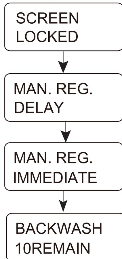
5. Once the valve is in the BACKWASH cycle, slowly open the inlet on the bypass valve to allow water to enter the unit. Let all air escape from the unit before fully opening the water supply. Allow the water to run to drain for 3–4 minutes, or until all media fines have been rinsed out and the drain water runs clear.
